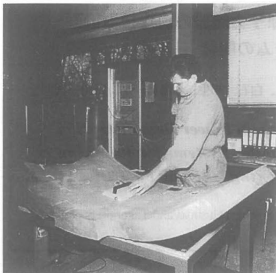
Photo 1 Clearance measurements for unrestricted reuse in Gundremmingen Power Station
