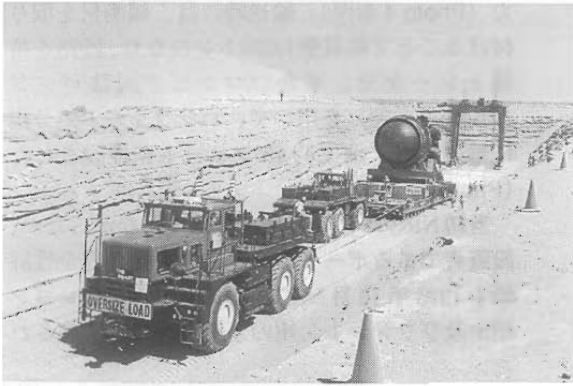
Photo 6 (Trojan) Unloading Work of Reactor Vessel and Internal Package at U.S. Ecology Disposal Site, Hanford
